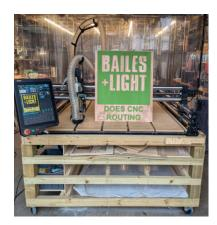
We have a Onefinity Elite CNC router. It has a 48" x 48" inch bed and a 18000RPM water-cooled spindle. It can cut sheet material up to 25mm thick.
