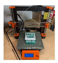
We run a Prusa Original i3 MK3S FDM 3D printer with a 0.4mm nozzle as standard. 0.25mm & 0.6mm nozzles are also available.
