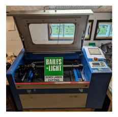
We have a 50W CO2 laser cutter capable of cutting thin material (<6mm) with a high degree of accuracy and only 0.5mm of <u>kurf</u>.
